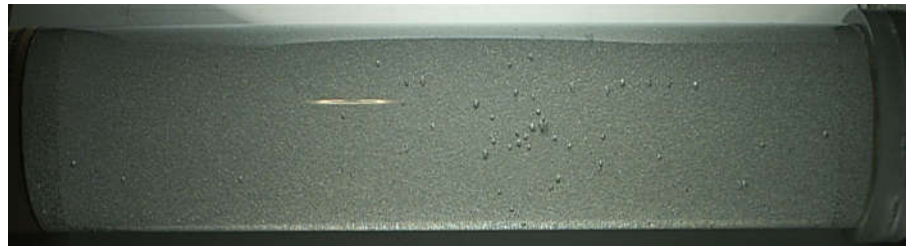
Fig.2 On the left the experimental apparatus with the sonotrode and the cavitation chamber at the centre, surrounded by the neutron bubble detectors. On the right the bubbles produced by the neutrons in one of the detectors. The position of the bubbles show some kind of tropism of the neutron emission (2006).
