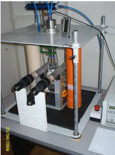
Fig.2 On the left the experimental apparatus with the sonotrode and the cavitation chamber at the centre, surrounded by the neutron bubble detectors. On the right the bubbles produced by the neutrons in one of the detectors. The position of the bubbles show some kind of tropism of the neutron emission (2006).
